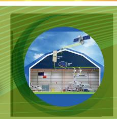
Global Foxcom's pioneering satellite phone repeater solution re-radiates satellite/GPS signals indoors, eliminating the need to step outside a building or underground facility for a clear line of sight. For avionic testing there is no need to take the aircraft out of the hangar, which saves on cost, time and the inconvenience due to inclement weather.
